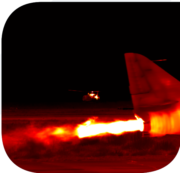
Jet Engine IR Signature Measurement
