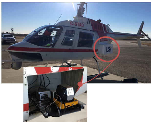
Figure 2. The Hyper-Cam Airborne Mini installed in a specially designed compartment at the rear of the Bell 206B helicopter used in the AMEP campaign. The instrument looks nadir through an opening at the base of the equipment bay.
