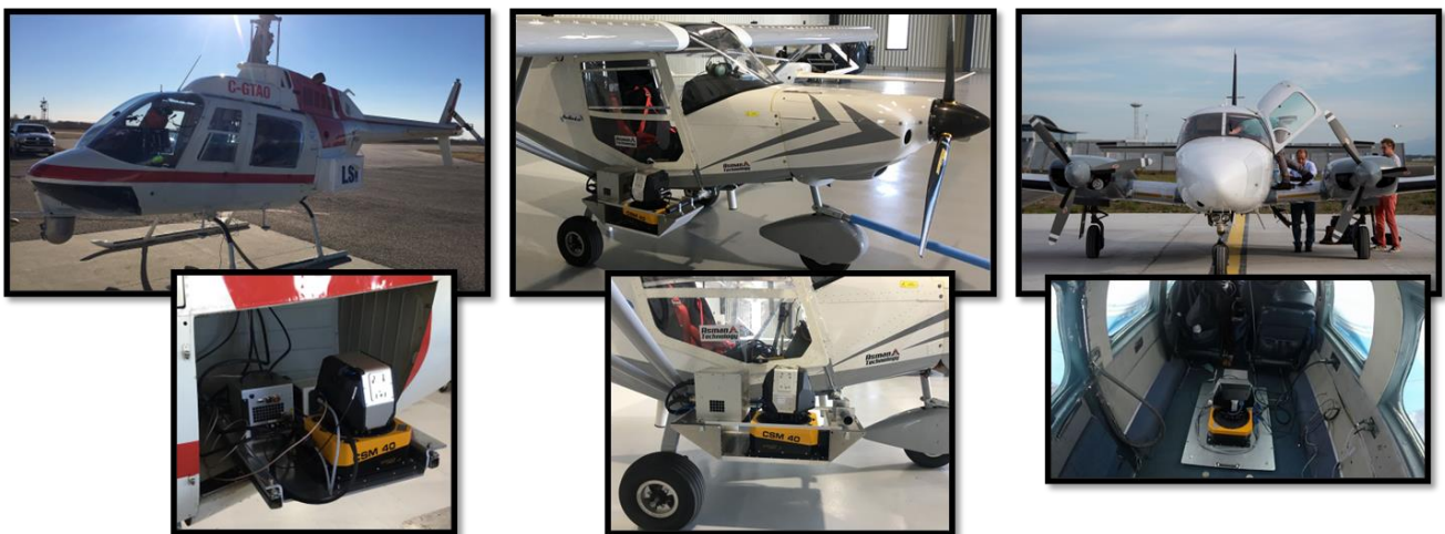
Figure 2: The Hyper-cam Airborne Mini has been integrated and used in various types of aircraft.
