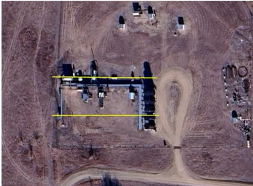
Figure 11: Example of Inspection Ground Lines (IGL) in yellow over a site to be inspected
