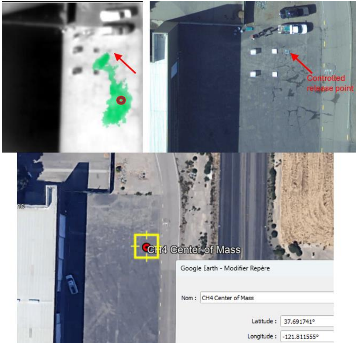
Figure 13: Emission source located within 0.5m using the high-resolution imagery of the Hyper-Cam Airborne Mini. Top-left image is the infrared image where pixels containing the methane are coloured in green. Top-right image is the visible image acquired at the same time as the infrared hypercube. The controlled release point is indicated. The bottom image is from Google Earth with the marker at the GPS coordinates of the centre of mass as reported in the detection report.
