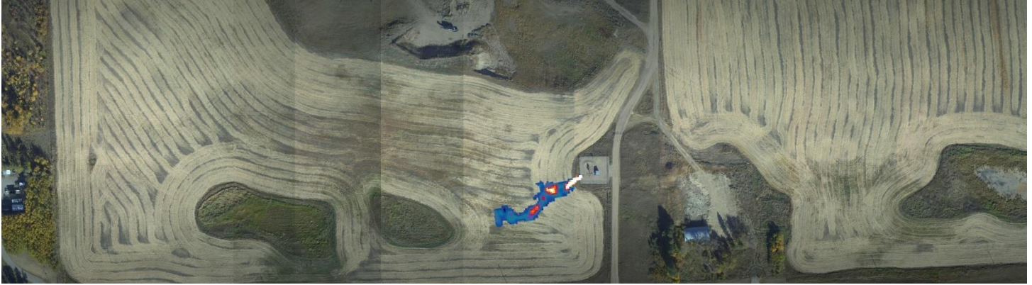
Figure 6. Methane gas leak observed with the Hyper-Cam Airborne Mini from a distance of 350 m. Methane plume color bar indicates gas concentration levels from low (blue) to high (yellow/white) path length concentration. To protect the privacy of our clients, the detected gas plume does not correspond with the location showed in the image.
