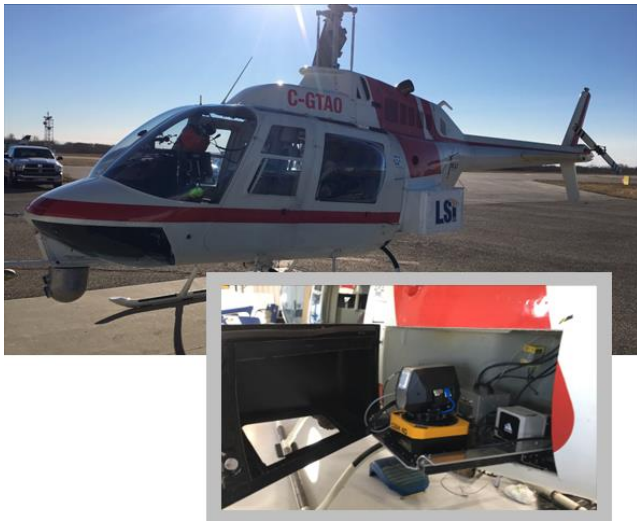
Figure 3. The Hyper-Cam Airborne Mini mounted on a Bell 206 helicopter to survey natural gas transmission lines.
