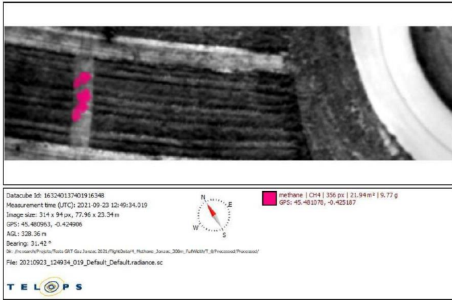
Figure 4. Example of a detection report produced by the system in real time. The methane plume is displayed in pink over the infrared image.
