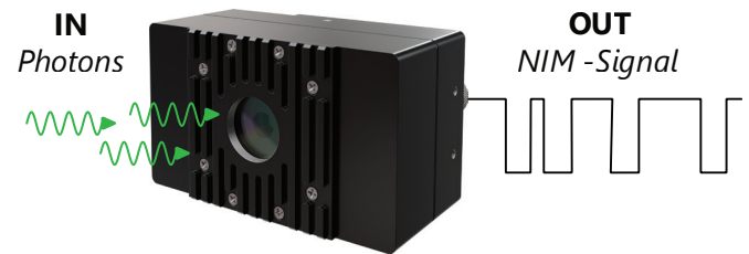
Figure 2: The PhotonPix™ converts the analog signal from the MCP-PMT to a digital NIM signal. This conversion determines the deadtime of the PhotonPix™. In this diagram the ultra short deadtime of under 1.6 ns is demonstrated. For the analog signal the peaks on the left with a time spacing of 0.8 ns only one digital signal is observed. When the time between two incidents photons increases to 1.6 ns, as shown on the right, two distinct signal are observed at the output.
