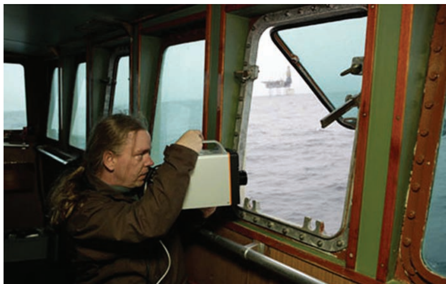
Figure 5. The high-resolution, high-sensitivity MWIR camera Onca performs a checkup from sea level.
