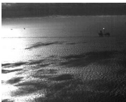
Figure 4. From above, methane plumes look like dark clouds in the MWIR spectrum.
