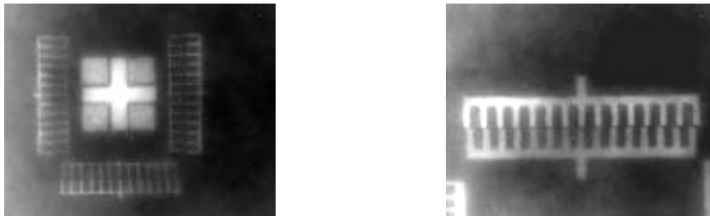
Fig. 1 SWIR images of alignment structures in a pair of bonded silicon wafers
