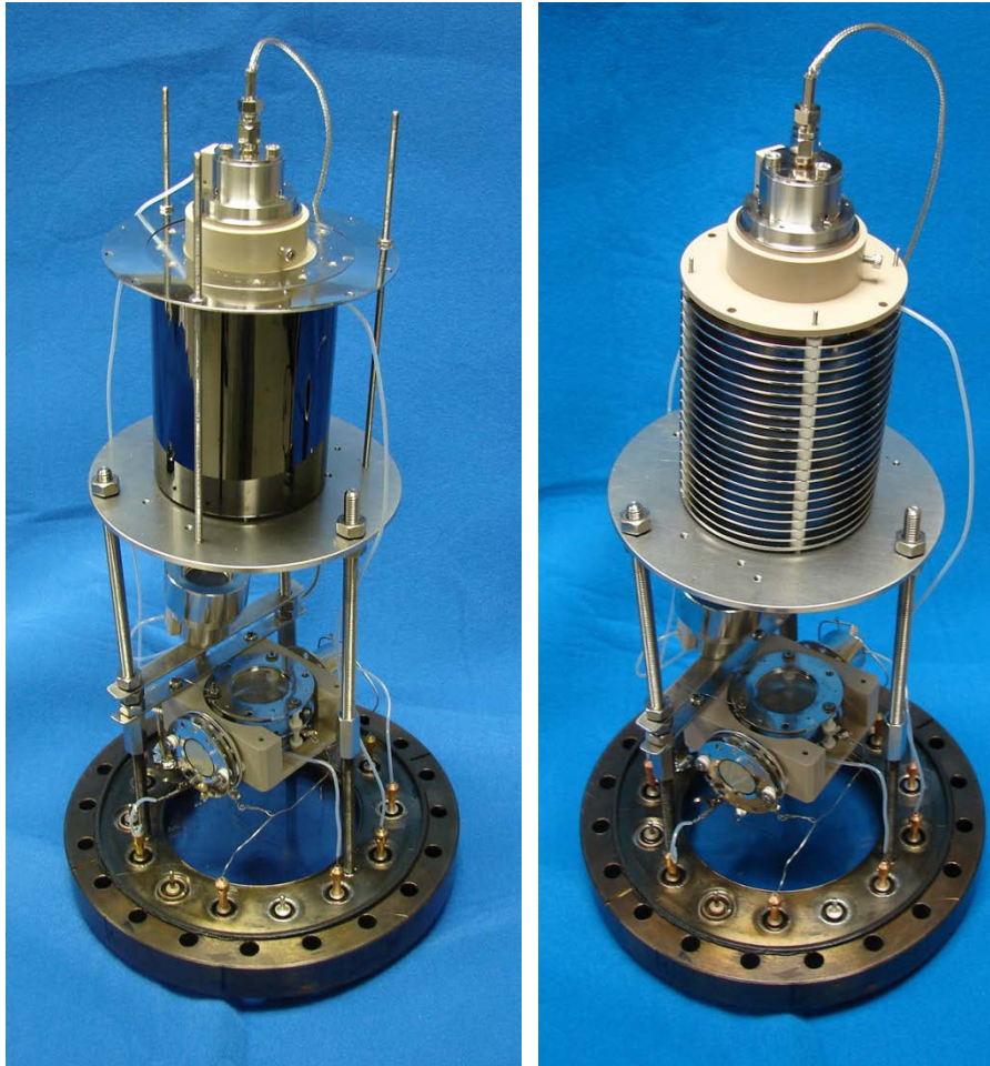
Figure 3: Resistive Glass and Stacked Ring Reflectron shown in place on experimental apparatus. The metal and glass reflectron could be interchanged without disturbing any of the other components.
