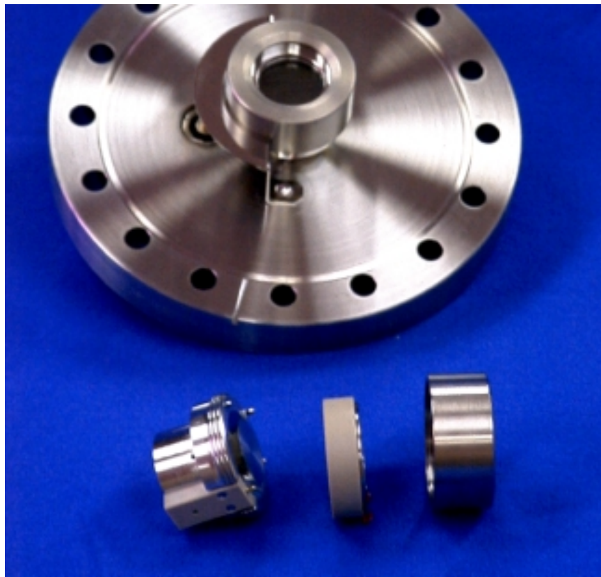
Figure 4 – The 2 micron pore MCP mounted in a Time-of-Flight Detector configuration
